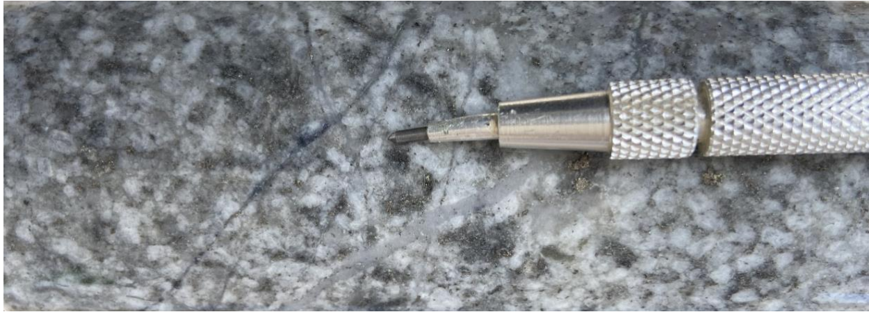
Figure 2. Drillhole LM24DD003 @ 315 metres. Close up of disseminated pyrrhotite-chalcocopyrite, pyrrhotite-chalcocopyrite – molybdenite veinlets and quartz- molybdenite veins.
