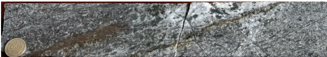
Figure 1. Drillhole LM24DD003 @ 300.75-301.30 metres. Pyrrhotite infill and stockwork of Early Biotite and quartz-chalcopyrite-molybdenite B veins.
